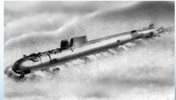
Artist concept of K-278 site. Note cracked hull & missing escape capsule (V-notch) in the sail
