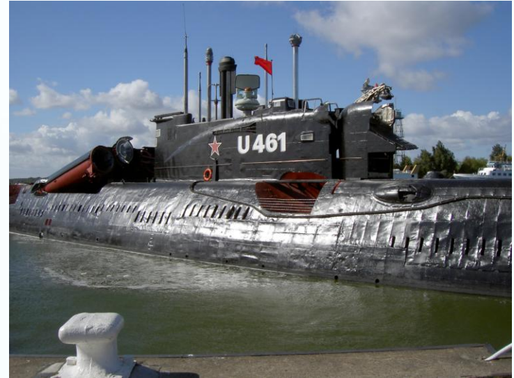
Elevated P-6 launcher & guidance radar in front of sail of a Juliett SS
