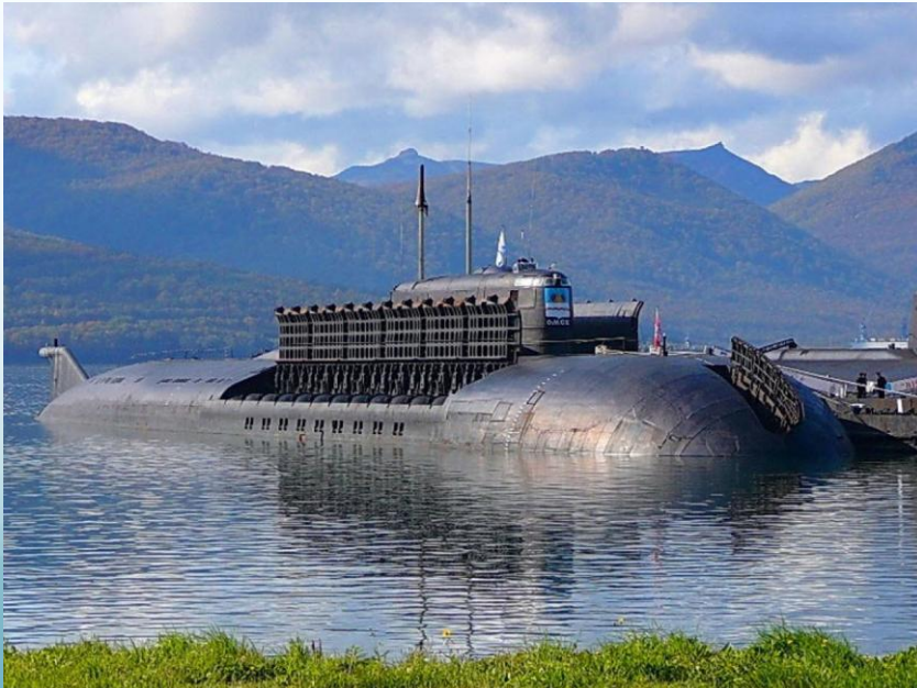
Oscar II-class SSGN Omsk with flank cruise missile hatches & bow torpedo loading hatch open
