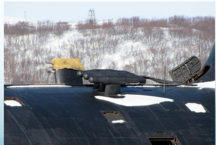
SOKS sensors on the outer hull casing, forward of the sail
