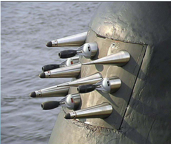
SOKS wake detection sensors on the leading edge of the sail
