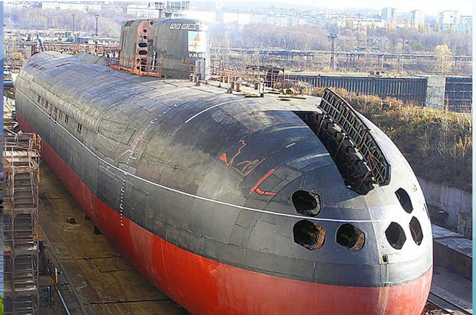
Oscar II-class SSGN Omsk in dry dock with bow torpedo loading hatch & torpedo tube doors open
