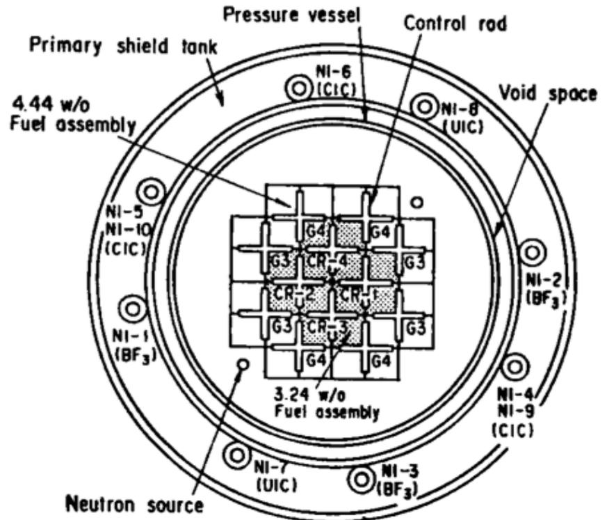
Mutsu reactor core cross-section
